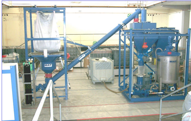
Continuously operated slurry mixer (1 t/h) at FZK
